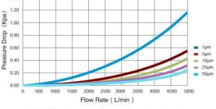
MFC BB Filter Pressure Drop vs.Flow Rate@20°C
